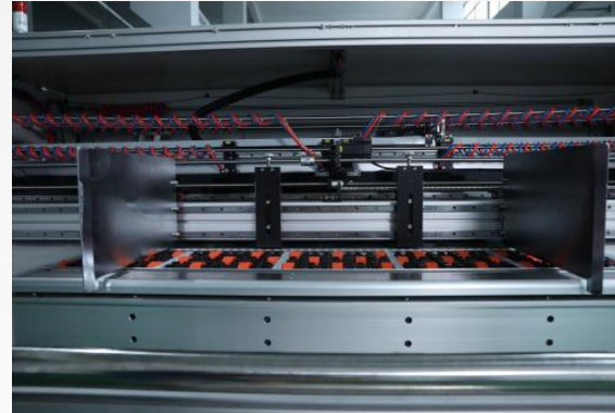
Continuous cardboard feeding system Leading edge feeder, 20~50 sheets can be loaded
