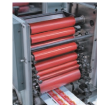
Superior ink transfer system 优越传墨系统
