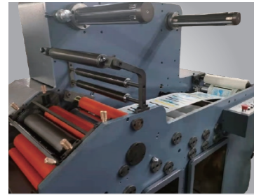
Continuous rewinder with UV vanish 连续收卷带光
